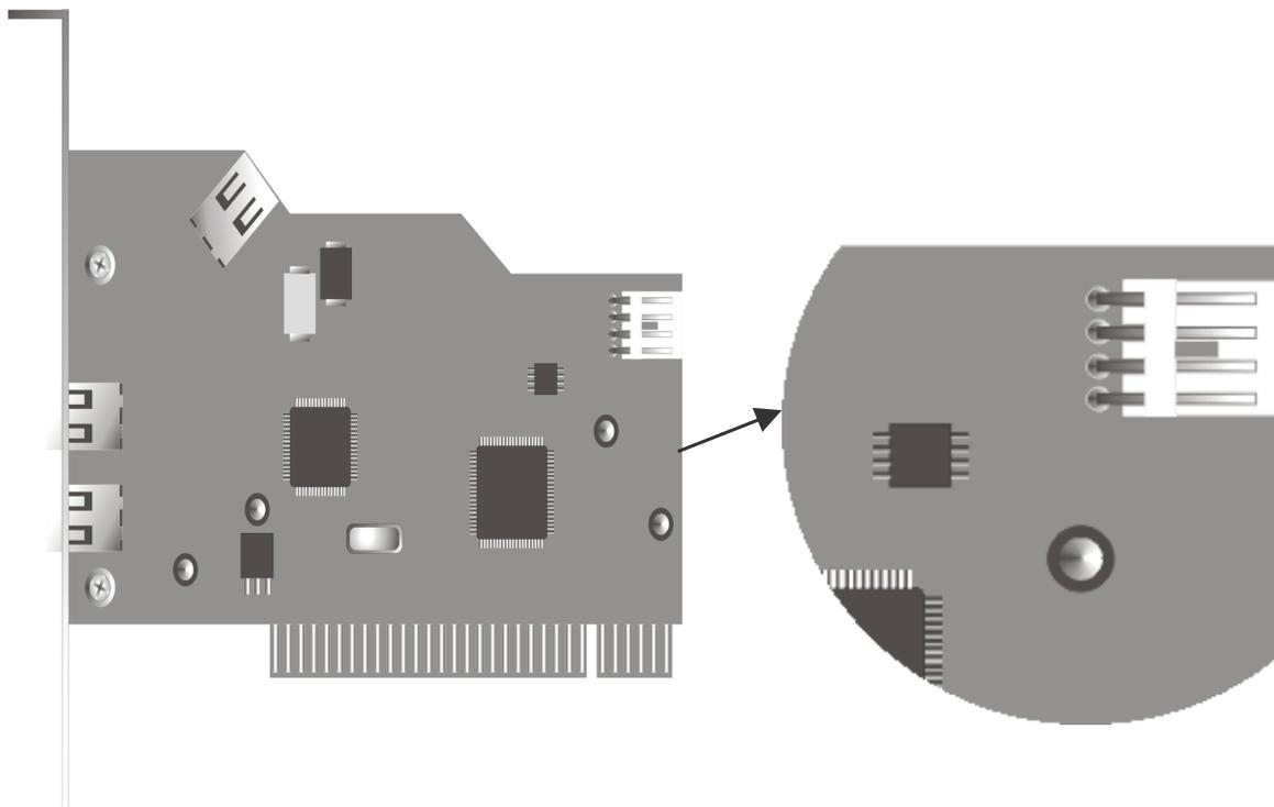
If you want to connect other IEEE 1394 devices that draw their power from the Cameo 400 DV at some time in the future, then you should connect the Cameo 400 DV directly to your PC power supply. This way the supply is not all drawn from the mainboard, eliminating overload on the PC electrical net.
