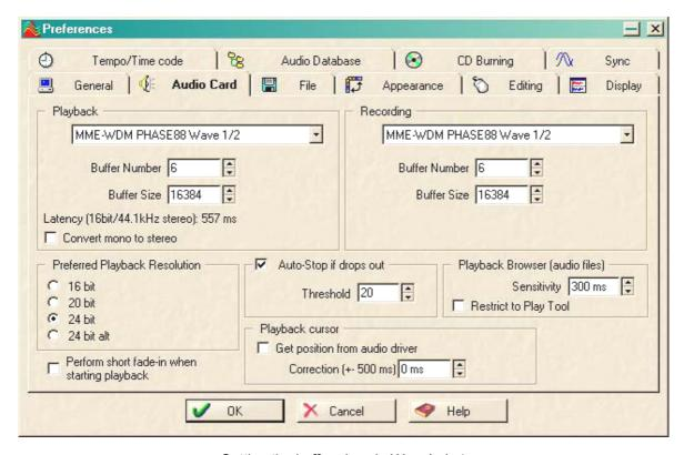
Setting the buffer sizes in WaveLab 4.
