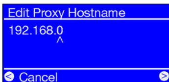
**5)** ... and enter the name (“proxy\_internet”) or the IP address. Use the following buttons: number buttons 1-9, 1 for the dots, Left/Right to move the cursor, and “Skip Back” to delete incorrectly entered characters. (s. chapter 3.1)
