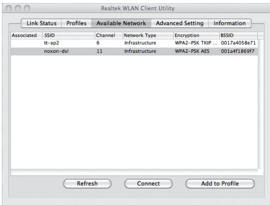
If the network is encrypted, you have to enter the corresponding WLAN key in the „Profile Properties“ input dialogue. Click OK to save and exit the setup of the NOXON WLAN Stick.
