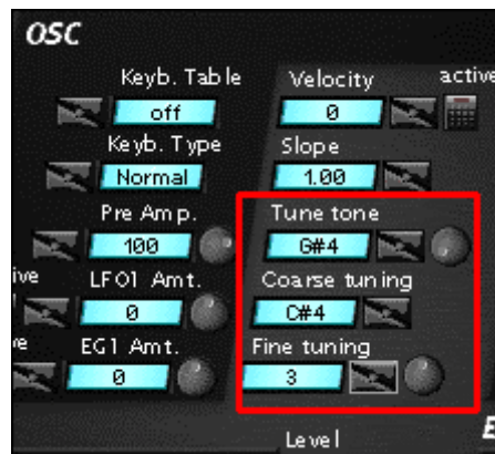
The OSC section contains the parameters for setting the root key and fine tuning.
